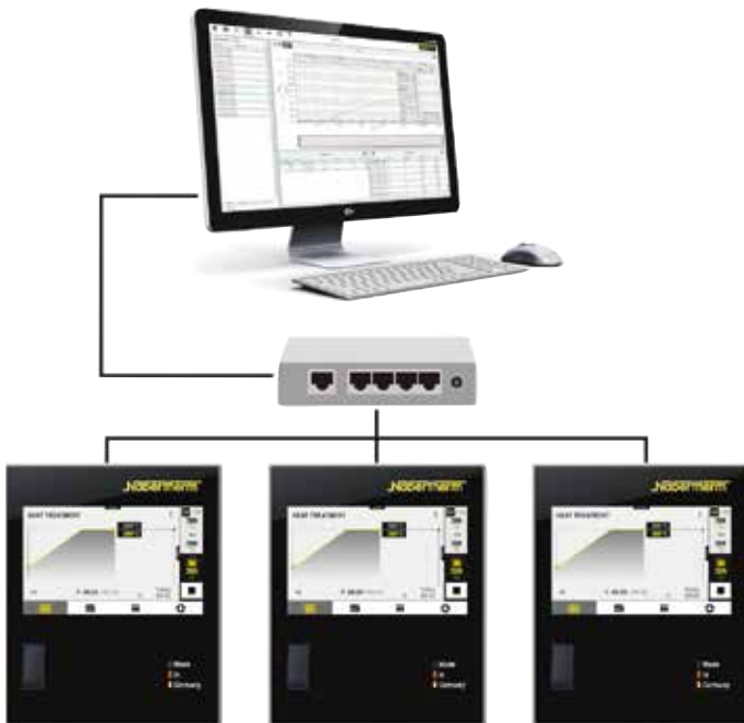
Example lay-out with 3 furnaces
