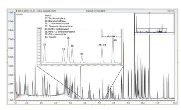
Figure 4. Total ion chromatogram (TIC) of a 5 ppb VOC standard (analyzed using the water method) with an inset indicating consistent peak shapes and separation with minimal water interference
