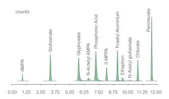
Figure 3. The typical chromatogram obtained after a 15 µL injection of 100 ppb standard solution on the Acclaim Trinity P1 column
