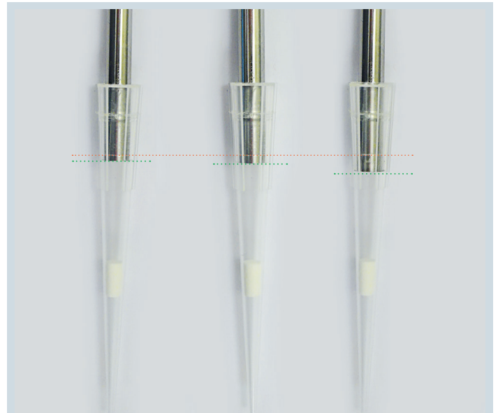
Fig. 5: Insertion depth of a testing prod in 20 µL tips of manufacturer G. All tips were taken from same box.
