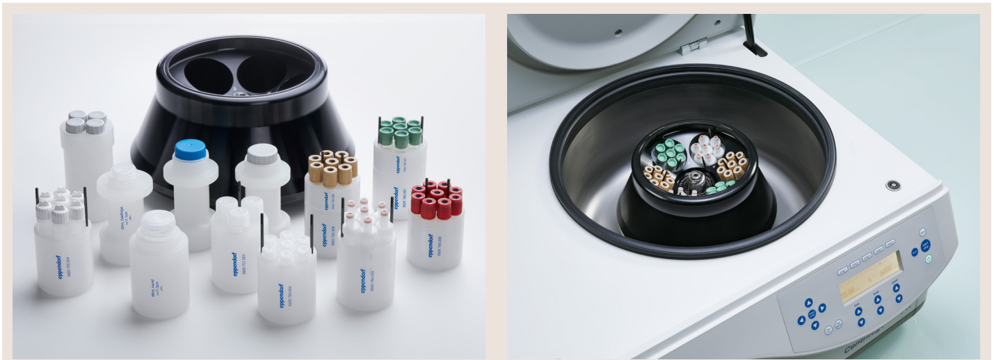
Figure 1: Rotor FA-6x250 is now extending the rotor range of the 59xx centrifuge family, offering a great flexibility in terms of vessels (e.g. 5/15/50 mL conical tubes, 10 – 85 mL Nalgene® oak ridge tubes, 13/16/17.5 mm blood collection vessels, FACS® tubes, ...) at a maximum speed of 15,054 x g . The patented and improved Dynamic Compressor Control technology in the 59xx centrifuges secures the best cooling performance for temperature sensitive applications like plasmid- or protein purification protocols.
