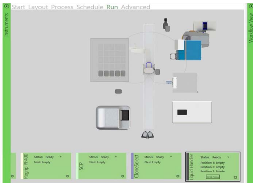
Figure 2. This virtual platform shows CSI-FL, automated incubator, liquid handler, hotel, and barcode readers. Integration of these instruments is done on a fully virtual environment (GBG) across a workstation to run an automated workflow. The devices were monitored in real-time and added or dropped off of the system based on the workflow needs.
