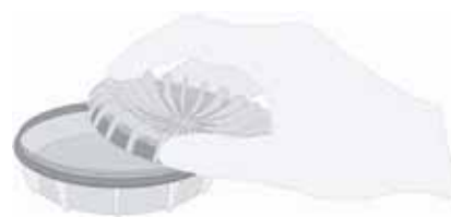
Concave lid can be used to scrape sample if stuck to the lid after the transport.
